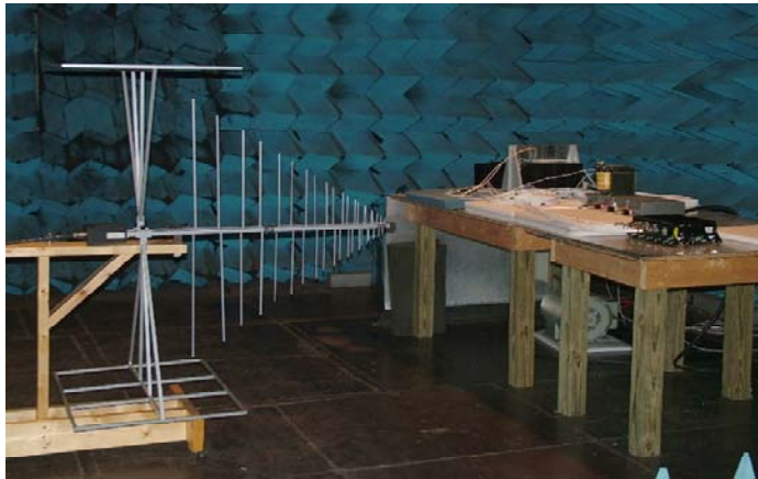
Radiated Emissions Test Setup
